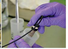
Fig.4 a, b & c: Measuring of pH and Redox (Eh) (Photo by HPC, 2014)
