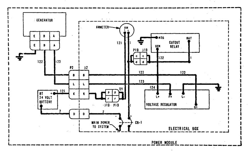
Figure I-1. Main Power Circuitry
