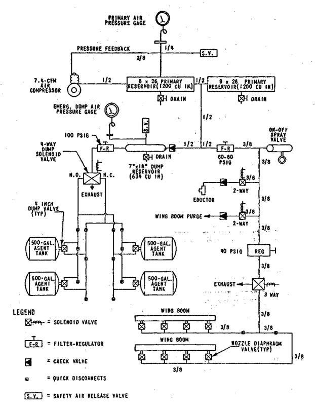
Figure 4. Pneumatic System Schematic
