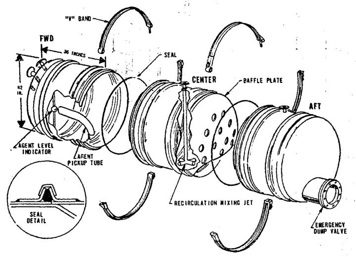
Figure 46. Tank Module (Original Concept)
