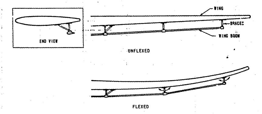
Figure 54. Dynamic Wing Boom Operation
