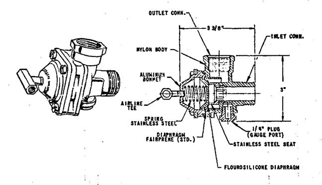
Figure 53. Nozzle Valve Assembly
