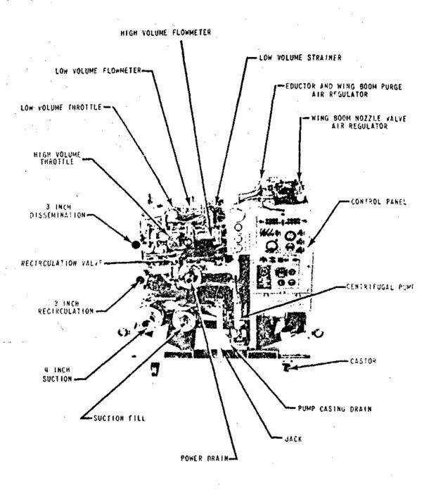
Figure 5. Power Module Assembly (Front View)
