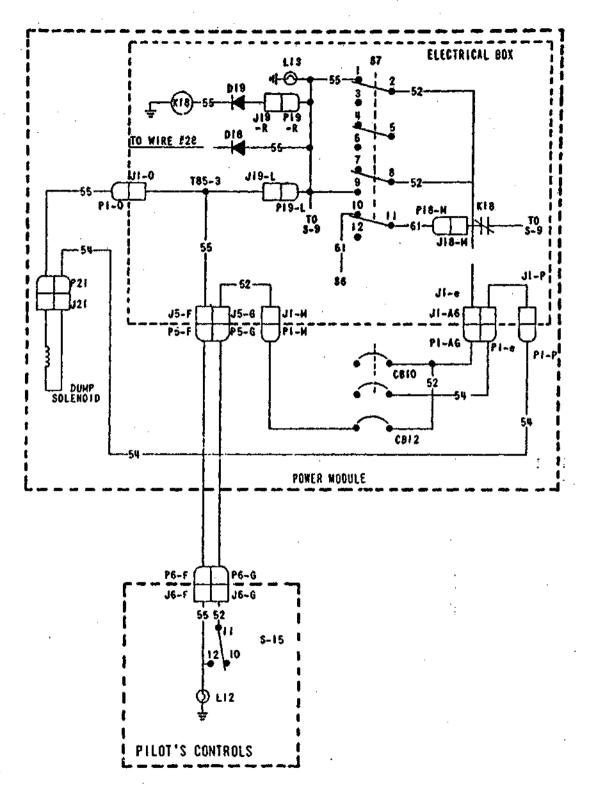
Figure I-8. Dump System Circuitry
