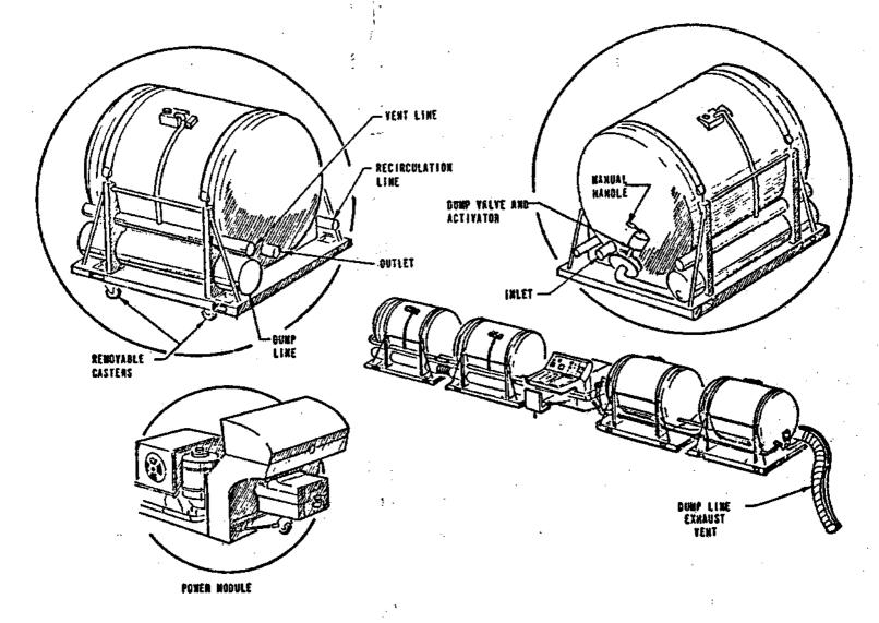
Figure 47. Split Series Tank Module (First Concept)
