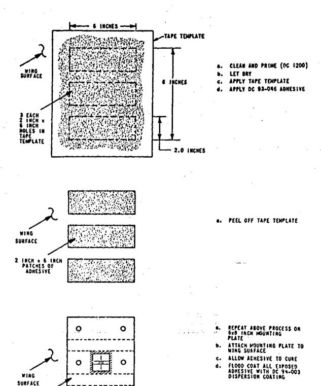
Figure 32. Modified Mounting Plate Design No. 4, Individual Bonding Pads
