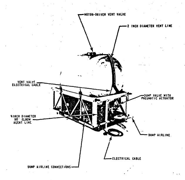
Figure 10. Tank Module Assembly (End View)
