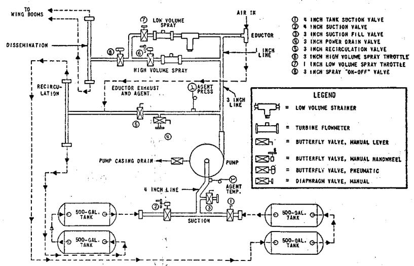
Figure 2.: Agent Transfer System Schematic
