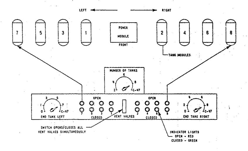
Figure 13. Vent Valve Control Schematic
