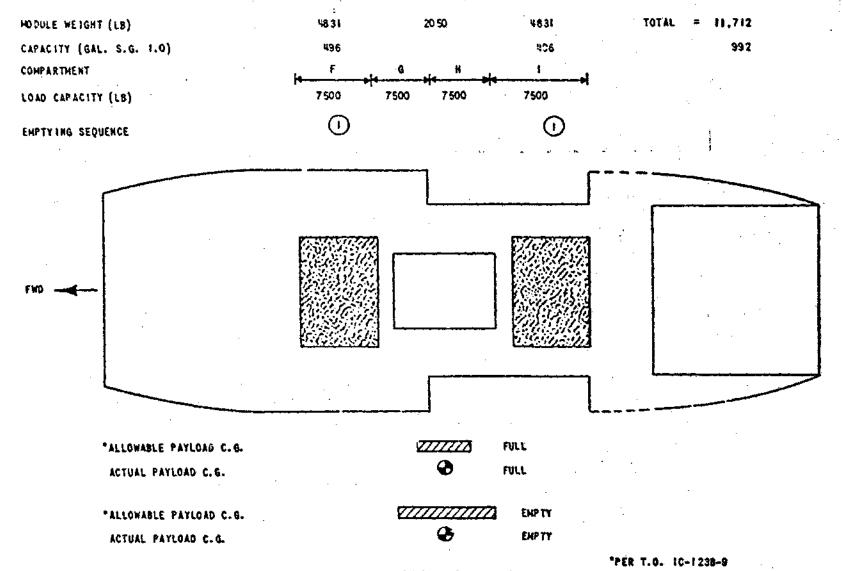
Figure 17. C-123K Floor Plan
