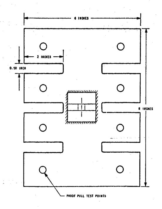
Figure 31. Modified Mounting Plate Design No. 3, Slotted Plate
