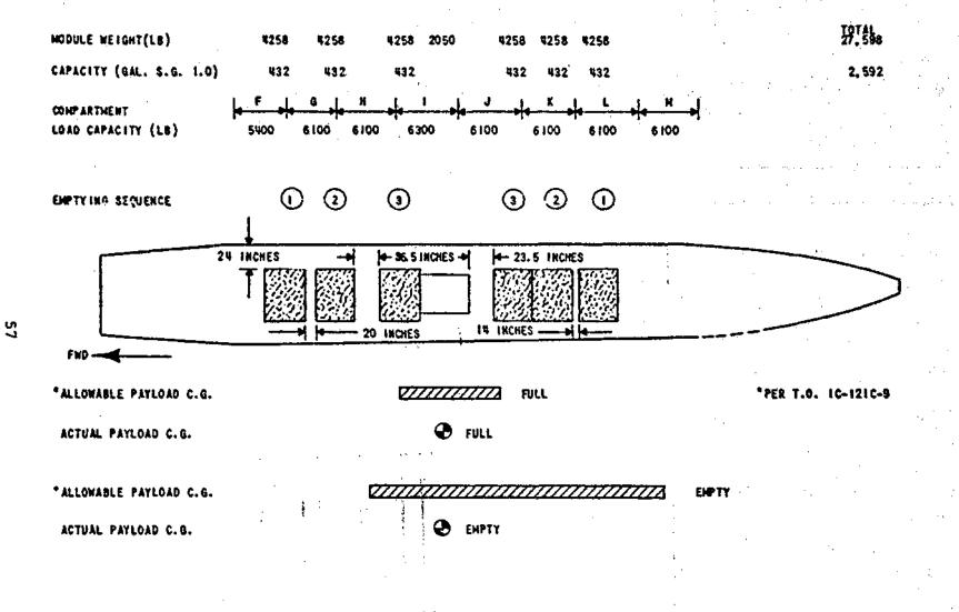
Figure 23. C-121G Floor Plan
