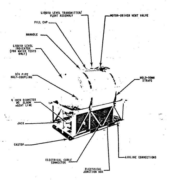
Figure 9. Tank Module Assembly (Side View)
