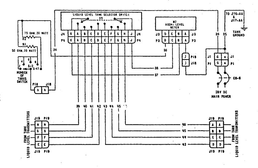
Figure I-5. Agent Level System Circuit
