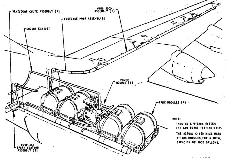
Figure 26. C-130 Modular Internal Spray System Kit No. 4374236
