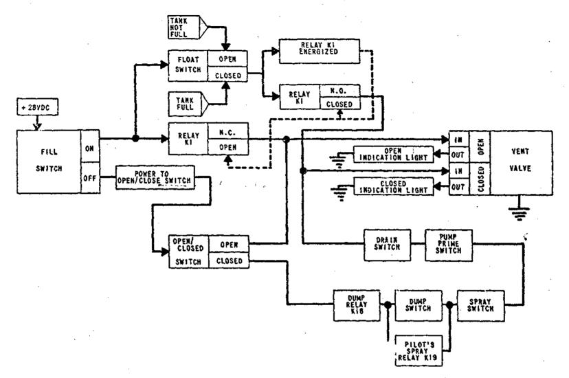
Figure 1-9. Vent Valve Control System Logic Diagram (One Valve)
