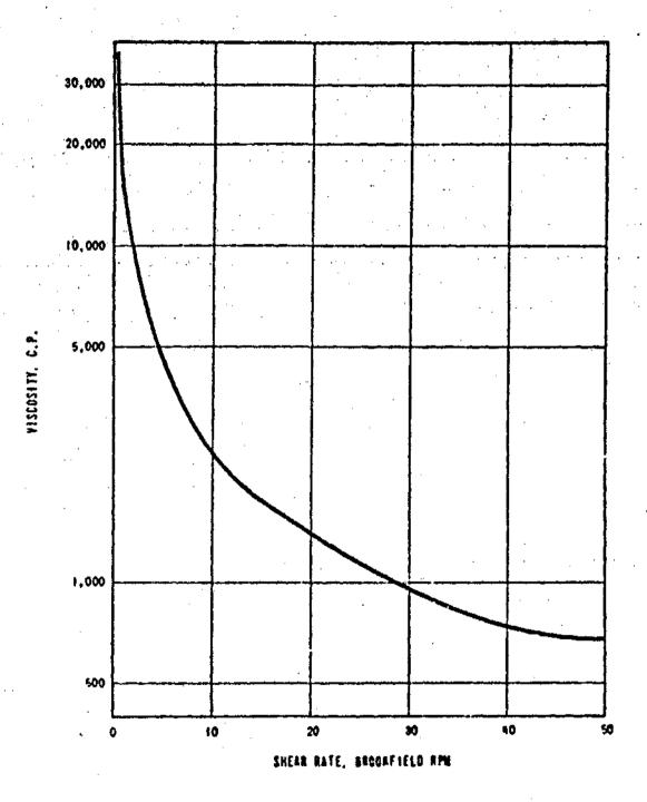
Figure 39. Thixotropic Nature of Slurried Fertilizer
