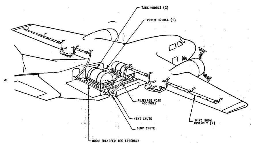
Figure 1. C-123 Modular Internal Spray System Kit No. 4373716
