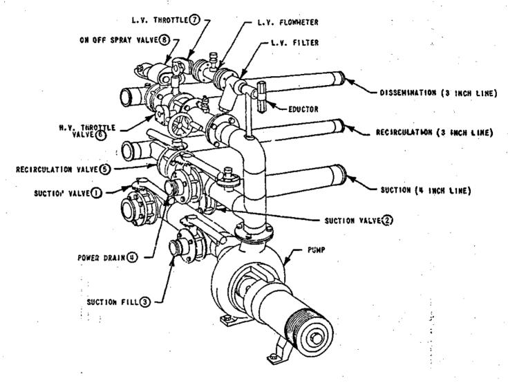
Figure 3. Agent Transfer System Power Module Piping
