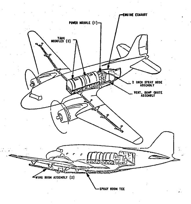
Figure 25. C-47 Modular Internal Spray System Kit No. 4374132
