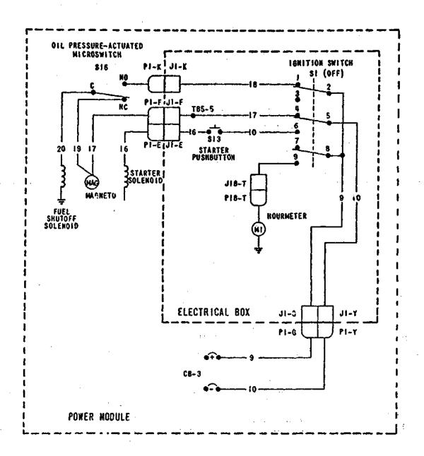
Figure I-4. Engine Control Circuit
