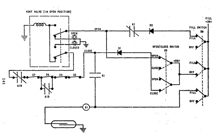
Figure I-10. Vent Valve Control System Schematic (One Valve)
