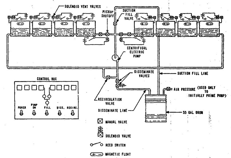
Figure 45. Plastic Flow Model Schematic
