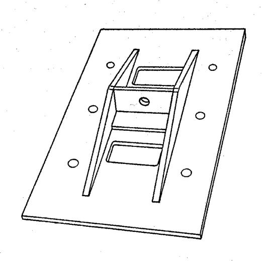
Figure 30. Modified Mounting Plate Design No. 2, Picture Frame with Gussets
