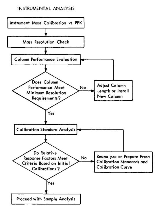
Figure 3. Daily QA procedures for proceeding with sample analysis.
