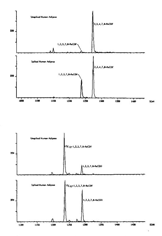
Figure 3. Example of the PeCDF (m/z 338) and PeCDD (m/z 354) HRGC/MS-SIM elution profiles in unspiked and spiked human adipose. The spiked concentrations for each isomer of PeCDF and PeCDD in these chromatograms were 25 pg/g.
