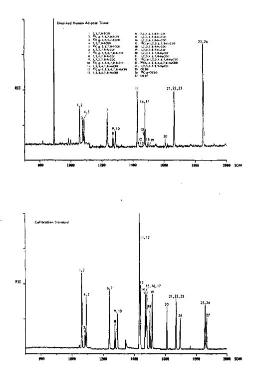
Figure 1. Comparison of the HRGC/MS-SIM reconstructed ion chromatogram (RIC) from the analysis of unspiked homogenized human adipose tissue matrix and a calibration standard for PCDDs and PCDFs.
