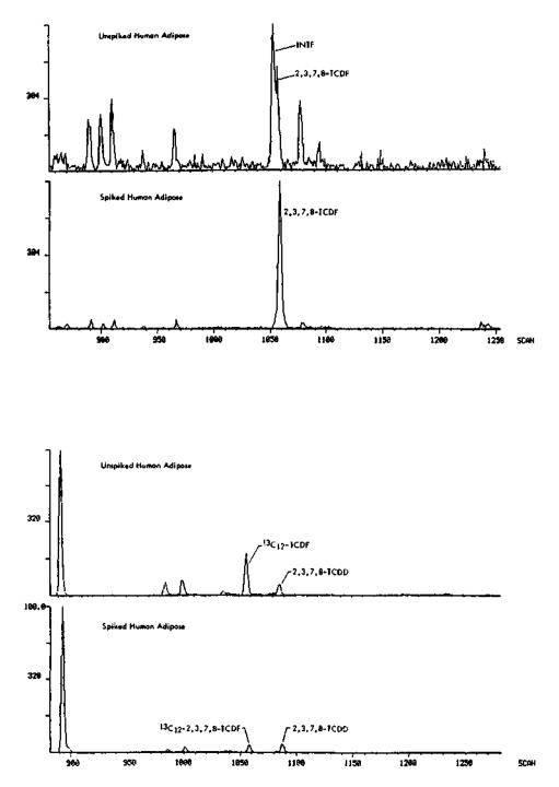
Figure 2. Example of the TCDF (m/z 304) and TCDD (m/z 320) HRGC/MS-SIM elution profiles in unspiked and spiked human adipose. The spiked concentrations for TCDF and TCDD in these chromatograms were 25 pg/g each.
