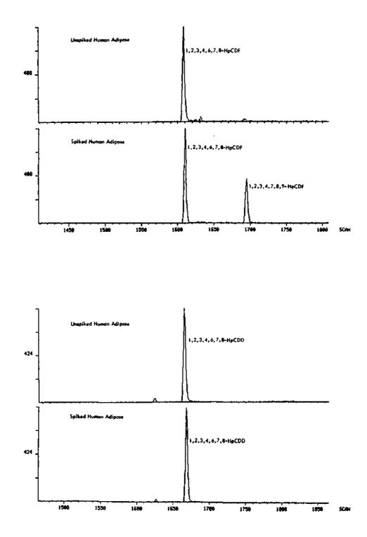
Figure 5. Example of the HpCDF (m/z 408) and HpCDD (m/z 424) HRGC/MS-SIM elution profiles in unspiked and spiked human adipose. The spiked concentrations for each isomer of HpCDF and HpCDD were 62.5 pg/g.
