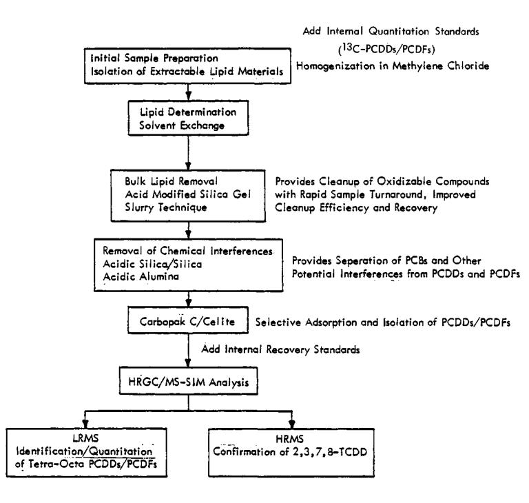
Figure 1. Schematic of the sample preparation and instrumental analysis procedures for determination of PCDDs and PCDFs in human adipose tissue.
