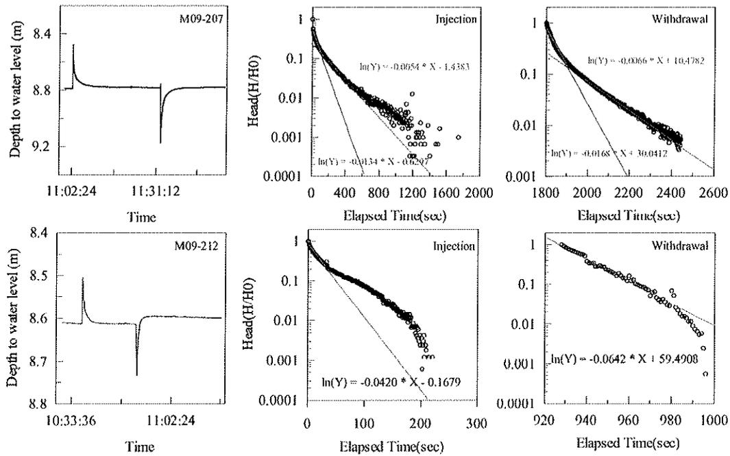
Figure 4 Curve-fitting results against elapsed time at constant slug tests in the B326.
