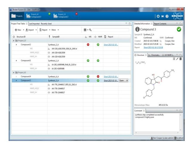
This new integrated solution for structure verification allows users to easily combine high-resolution accurate-mass (HRAM) mass spectrometry (MS), and complementary Nuclear Magnetic Resonance (NMR) data. FUSION-SV
