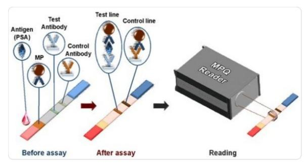
The antigen is the test protein (e.g. PSA). MP is the magnetic nanoparticle, the upside down Y is the antibody to the test protein. The test antibodies (the blue Ys) capture the test protein, and the control antibodies (the yellow Ys) capture the antibodies with the nanoparticles.
