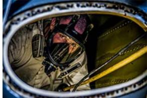
Airman 1st Class Nicholas McKinney prepares to be extracted from the inside of a C-17 Globemaster III fuel tank during training at Joint Base Charleston, S.C. Fuel system repair airmen remove, repair and install the fuel cells and tanks. (*Photo by Airman 1st Class Tom Brading*)
