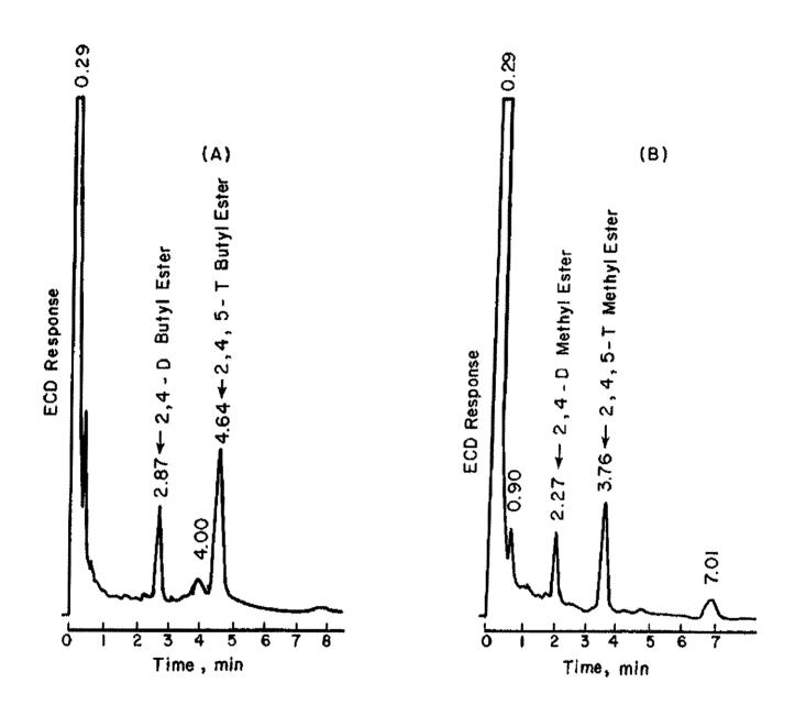
FIGURE 26. GC CHROMATOGRAMS OF (A) CHROMOSORB SAMPLE CD 29Y707J AND (B) WATER SAMPLE WS 30Y700J
