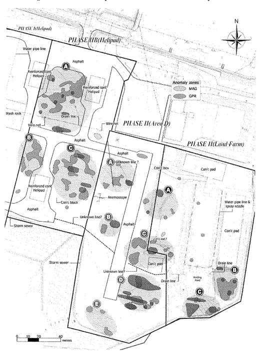
Figure 1-3. Final Interpretation of Subsurface Anomaly Zones
