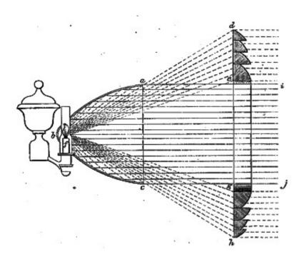
Figure 2. Argand's Lamp with Parabolic Reflector and Fresnel Lens Panel<sup>22</sup>
