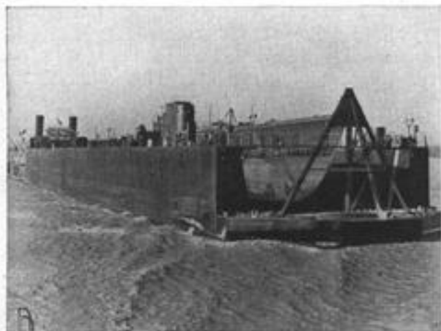
SUBMARINE, built in Wisconsin, was ferried down the Mississippi in a floating drydock pushed by riverboat.
