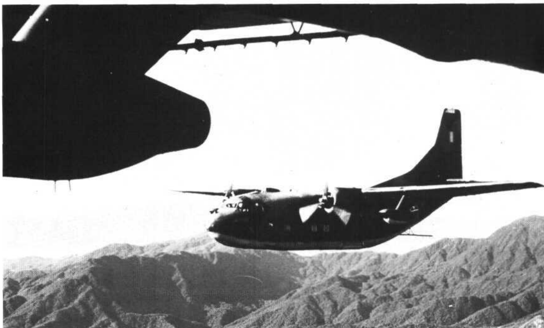
Fig. II B-2. UC-123 aircraft showing wing and tail spray booms. Photo taken in 1969 by Colonel Harold C. Kinne, Jr.
