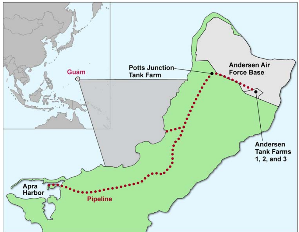
Figure 11: Fuel Pipeline from Naval Base Guam to Andersen Air Force Base in 1968
