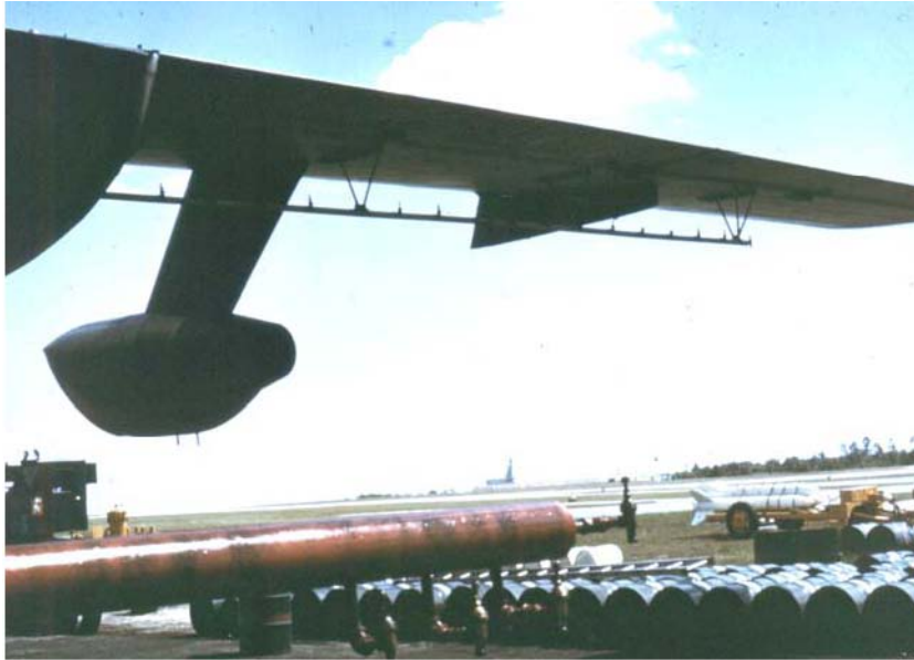
Figure 6.11 A wing defoliation spray boom mounted on the UC-123K aircraft at Hardstand 7 in 1969; note drums of Agent White and the Eglin AFB Airdrome in the background (Photograph courtesy of AFATL, Eglin AFB, Florida)
