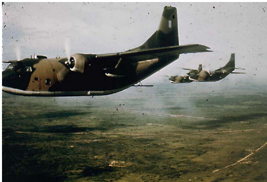
Figure 3.6 The UC-123K "Provider" with its Modular Internal Spray System was the "workhorse" for RANCH HAND. This high-wing, twin-engine assault transport had excellent low speed maneuverability, and the high-mounted wings allowed convenient positioning of wing spray booms. Note the spray boom mounted aft of the cargo door and
