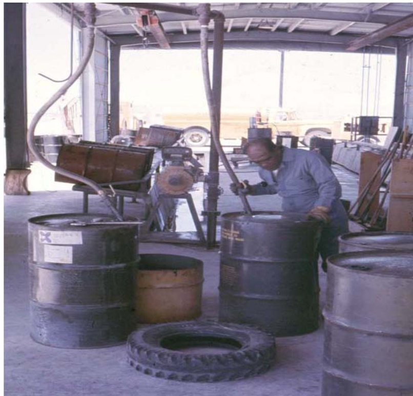
Figure 4.25 Removing drum lids prior to the contents (Agent Orange) being removed by a suction wand, Operation PACER HO, Naval Construction Battalion Center, Gulfport, Mississippi 24 May - 10 June 1977 (Photograph courtesy of USAF OEHL, Brooks AFB, Texas)
