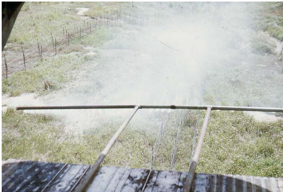
Figure 3.22 A photograph of the base perimeter of Phan Rang Air Base at the time of aerial application of Agent Blue by the use of a modified spray rig mounted in the cargo bay and door of a C-7. Notice the “in-depth” wire fencing (i.e., two rows consisting of three lines of fence, each one meter apart). Because the base bordered civilian dwellings, this fence arrangement was intended to keep civilians from inadvertently entering base perimeter areas (photograph courtesy of US Army Chemical Corps)
