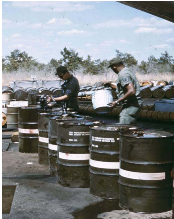
Figure 6.12 Air Development and Test Center (ADTC) personnel adding Methylene Blue Dye to Agent White prior to a mission on Test Area C-52A, Eglin AFB, Florida, 1969 (Photograph courtesy of AFATL, Eglin AFB, Florida)
