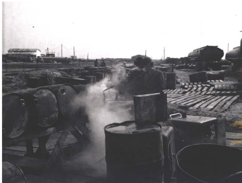
Figure 4.10 Usable empty Agent Orange drums were steam cleaned and provided to the Vietnamese Air Force (VNAF), Operation PACER IVY, Da Nang Air Field, 15 January 1972 (Carmichael Journal 1972)
