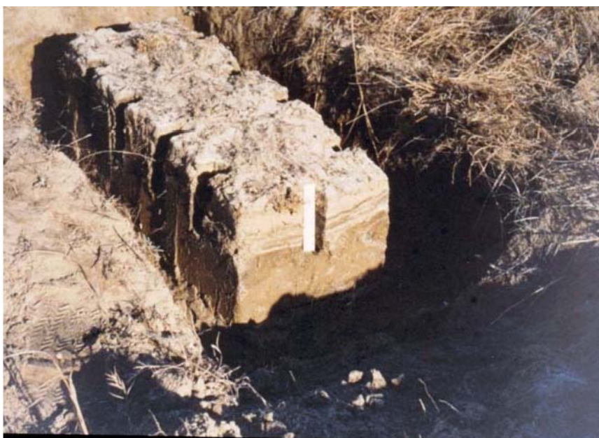
Figure 6.43 The methodology for collecting soil cores for TCDD analysis in 1974 and 1978, Test Area C-52A, Eglin AFB, Florida (Photograph courtesy of A.L. Young)
