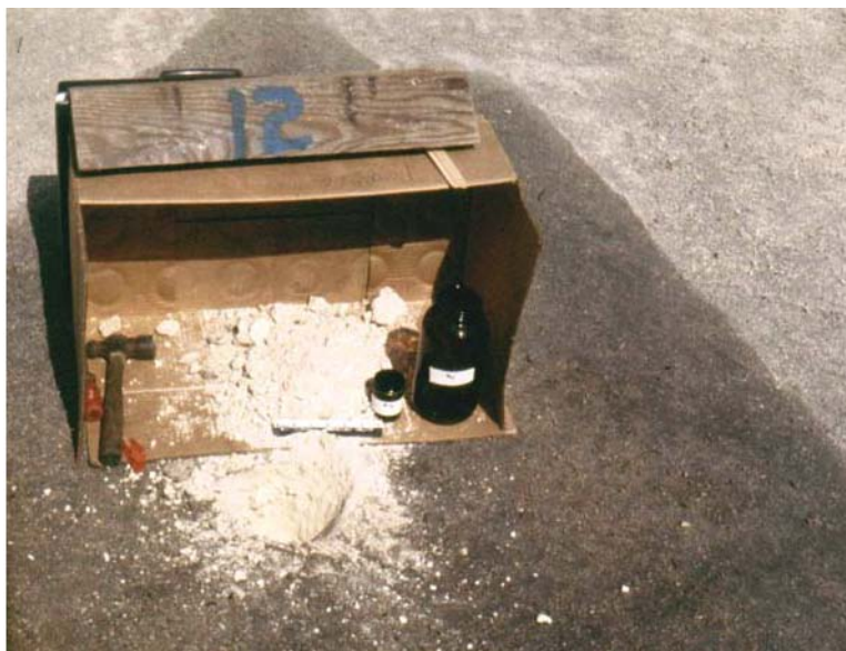
Figure 7.9 A photograph of Sampling Site Number 12 on Johnston Island, 25 August 1977. Note that the coral was so compacted that a hammer and chisel were required to collect the sample; a numbered metal stake was placed in the approximate center of the spill for identification for future sampling (Photograph courtesy of A.L. Young)
