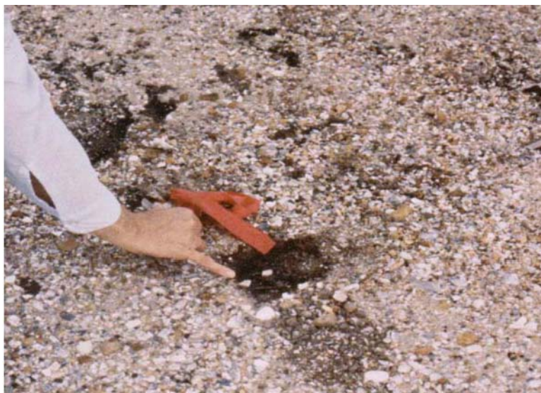
Figure 7.8 A photograph of a sampling site for herbicide residue from the former Herbicide Orange Storage Site at NCBC in July 1977. Note that the oyster shells were removed before the soil sample was obtained. The sample was collected 15 cm from a numbered metal stake (Photograph courtesy of A.L. Young)
