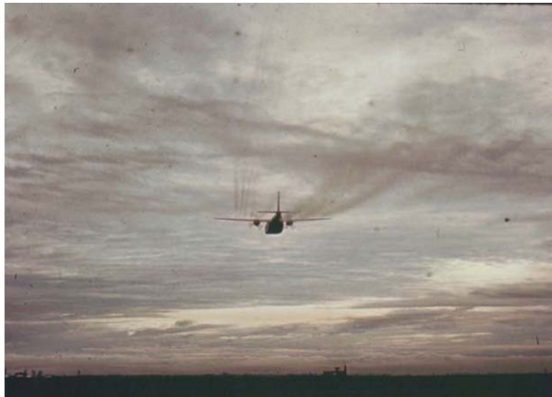
Figure 6.2 C-123B RANCH HAND aircraft conducting a Test and Evaluation Flight of the MC-1 Defoliant Spray System, Test Area C-52A, Eglin AFB, Florida, 1963 (Photograph courtesy of the AFATL, Eglin AFB, Florida)
