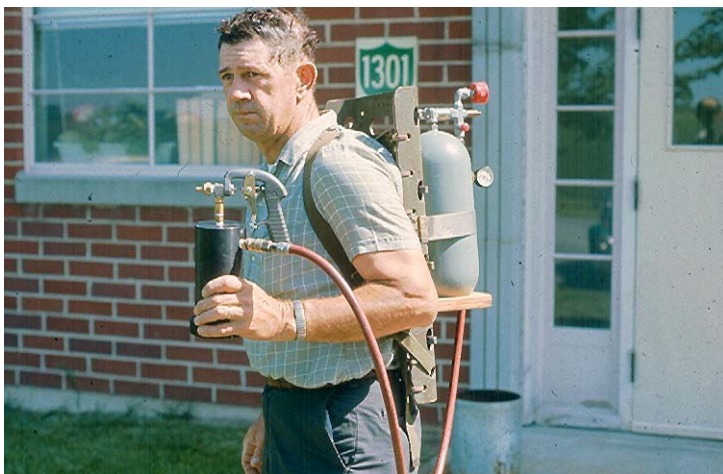
Figure 2.2 A 1970 photograph of the hand applicator used in the initial defoliant screening tests at Fort Detrick. The sprayer was a specially calibrated unit capable of delivery less than 0.1 kg/ha of candidate defoliants (photograph courtesy of A. Young)
