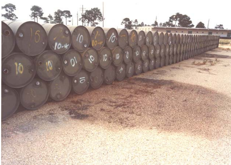
Figure 7.5 A photograph taken at NCBC on June 1975 showing the soil contamination initiated by a "pinhole" size leak in a drum of Agent Orange identified by an Analysis Sequence Number 10 (ASN 10), as a product produced by The Dow Chemical Company, and found to have a TCDD mean concentration of 0.25 ppm (Photograph courtesy of AFLC, Kelly AFB, Texas)
