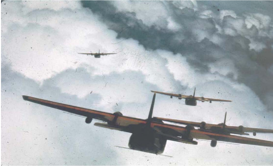
Figure 3.19 A photograph of four UC-123K aircraft “heading down” to the target. Note the bright red band across the upper surface of the wings. This was so FACs and fighters could more easily see the camouflaged RANCH HAND aircraft when at tree-top level. The photograph was taken over II Corps, 23 August 1969 (Photo courtesy of J. Ray Frank, Frederick, Maryland)
