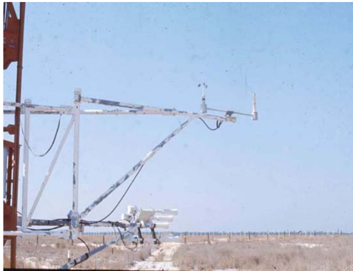
Figure 6.6 Sampling array for wind, temperature, and droplet dispersal data on the 90-meter tower in the center of Test Area C-52, Eglin AFB, Florida, 1969 (Photograph courtesy of A.L. Young)
