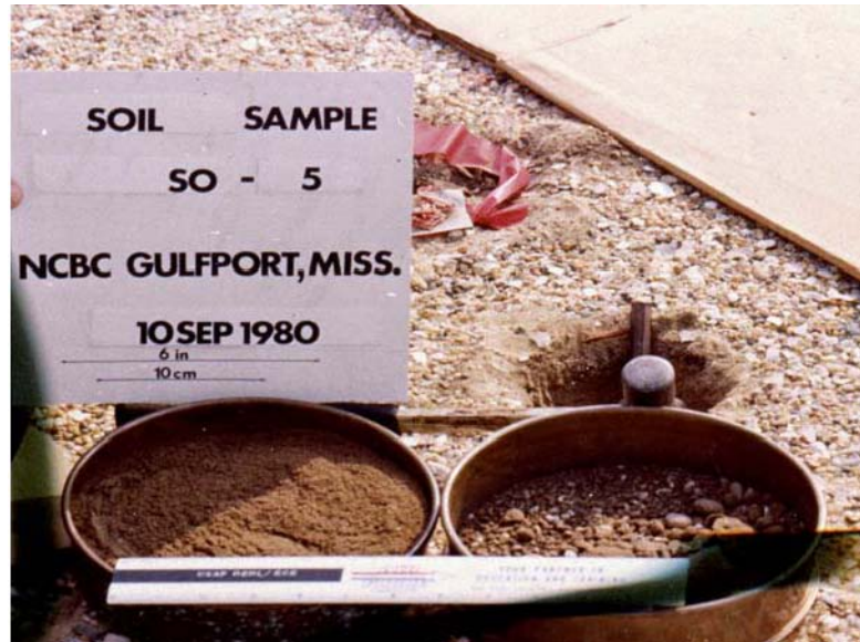
Figure 7.17 A photograph taken 10 September 1980 by personnel from the Engineering Services Laboratory showing the sampling protocol for collecting soil samples on the former Herbicide Orange Storage Site, NCBC (Photograph courtesy of AFESL, Tyndall AFB, Florida)
