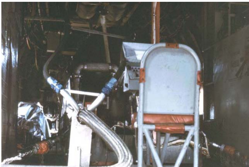
Figure 6.10 An interior view of the A/A 45 Y-1 Internal Modular Spray System mounted in the UC-123K aircraft, Hardstand 7, Eglin AFB, Florida 1969 (Photograph courtesy of AFATL, Eglin AFB, Florida)
