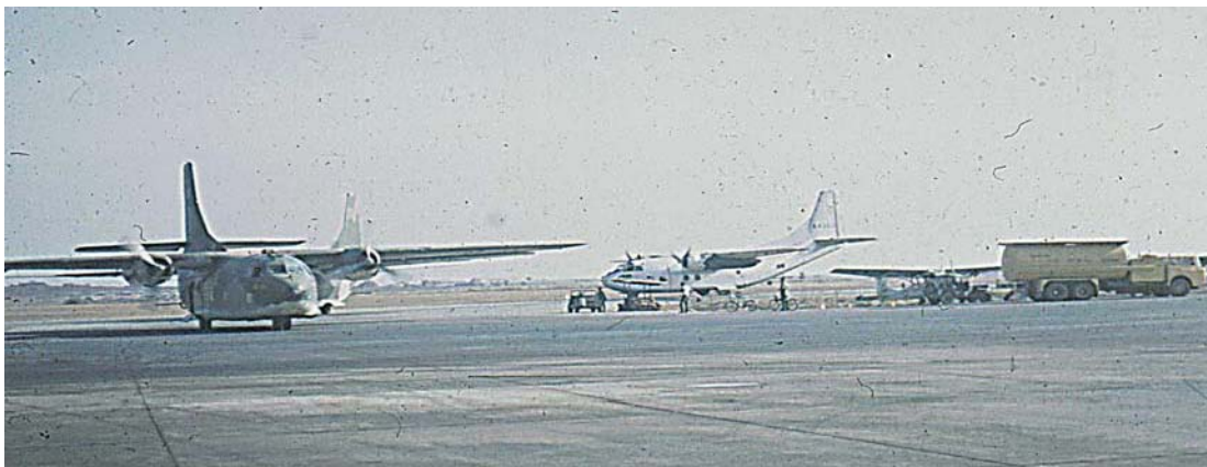
Figure 3.28 Photographs of “Silver Bug Birds” which were RANCH HAND UC-123 aircraft dedicated to the spraying of malathion insecticide for mosquito control. Each aircraft could spray more than 6,000 hectares and routinely treated 14 bases and their adjacent Vietnamese cities every nine days. Re-servicing was available at the air bases at Cam Ranh Bay, Bien Hoa and Da Nang (Photographs courtesy of J. Ray Frank, Frederick, Maryland)
