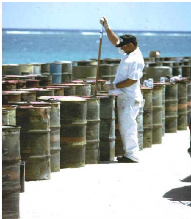
Figure 5.2 Sampling drums of Agent Orange for Dioxin content, 1973, Johnston Island. A random sample of 200 drums was assumed to represent a population of 25,220 drums
