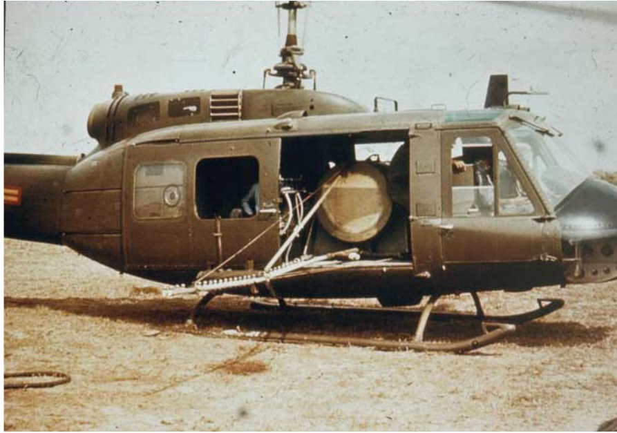
Figure 3.7 The Military UH-1 series of helicopters generally sprayed the herbicides. The most common spray systems were the HIDAL and AGRINAUTICS units. They could be removed from the aircraft in a matter of minutes. Each unit consisted of a 760-liter tank and a collapsible 9.8-meter spray boom (Photograph courtesy of the US Army Chemical Corps)
