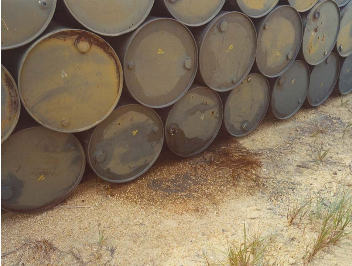
Figure 7.4 A photograph of a leaking drum in June 1975 within the NCBC Herbicide Orange Inventory (Photograph courtesy of AFLC, Kelly AFB, Texas)
