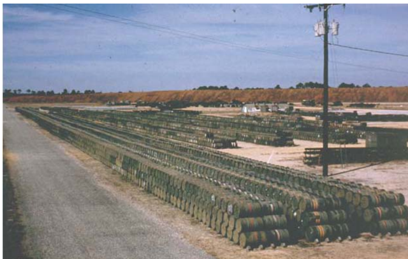
Figure 4.22 Photograph of the Agent Orange inventory in 1974, at the Naval Construction Battalion Center; the inventory was initially stored upright on pallets, but the drums were subsequently placed on their sides on wooden dunnage (Photograph courtesy of AFLC, Kelly AFB, Texas)
