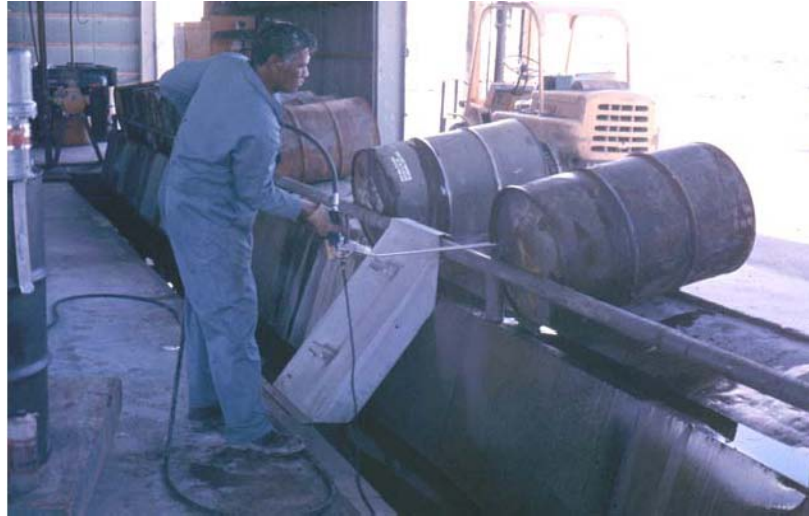
Figure 4.26 Draining and rinsing Agent Orange drums, Operation PACER HO, Naval Construction Battalion Center, Mississippi, 24 May - 10 June 1977 (Photograph courtesy of USAF OEHL, Brooks AFB, Florida)
