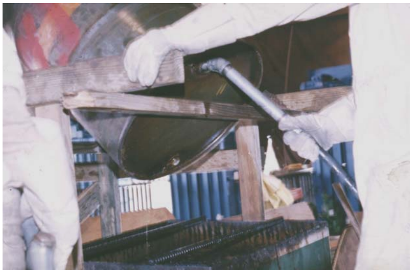
Figure 4.19 De-drumming and rinsing operation of an Agent Orange drum at Naval Construction Battalion Center, Gulfport, MS, April 1975; a full-time crew was required to maintain oversight of the inventories at NCBC and Johnston Island (Photograph courtesy of AFLC, Kelly AFB, Texas)
