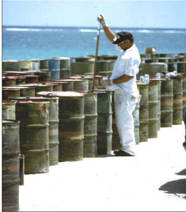
Figure 5.2 Sampling drums of Agent Orange for Dioxin content, 1973, Johnston Island. A random sample of 200 drums was assumed to represent a population of 25,220 drums (Photograph courtesy of USAF OEHL, Brooks AFB, Texas)
