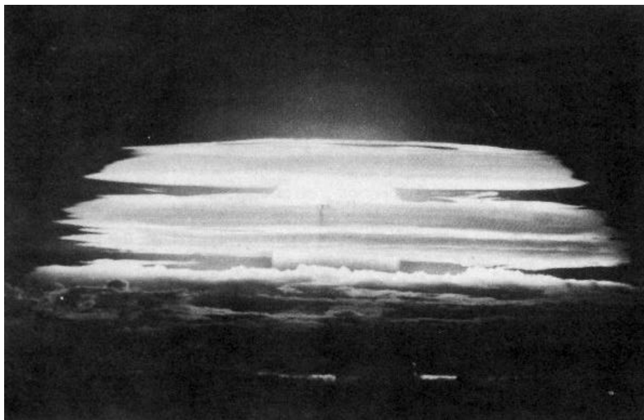
Figure 2.04 Fireball from an air burst in the megaton energy range, photographed from an altitude of 12,000 feet at a distance of about 50 miles. The fireball is partially surrounded by the condensation cloud.
