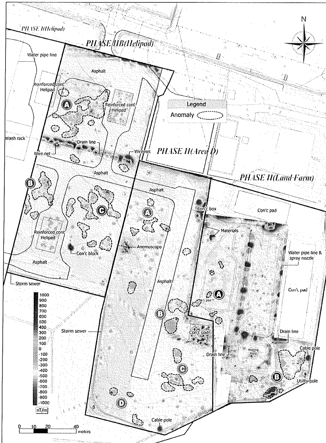
Figure 3-1. Magnetic Gradiometry Survey Result
