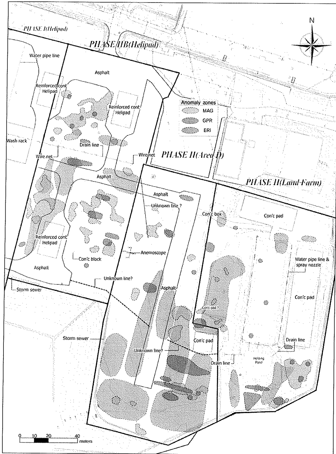
Figure 4-4. Combined Magnetic Gradiometry, GPR and ERI Results
