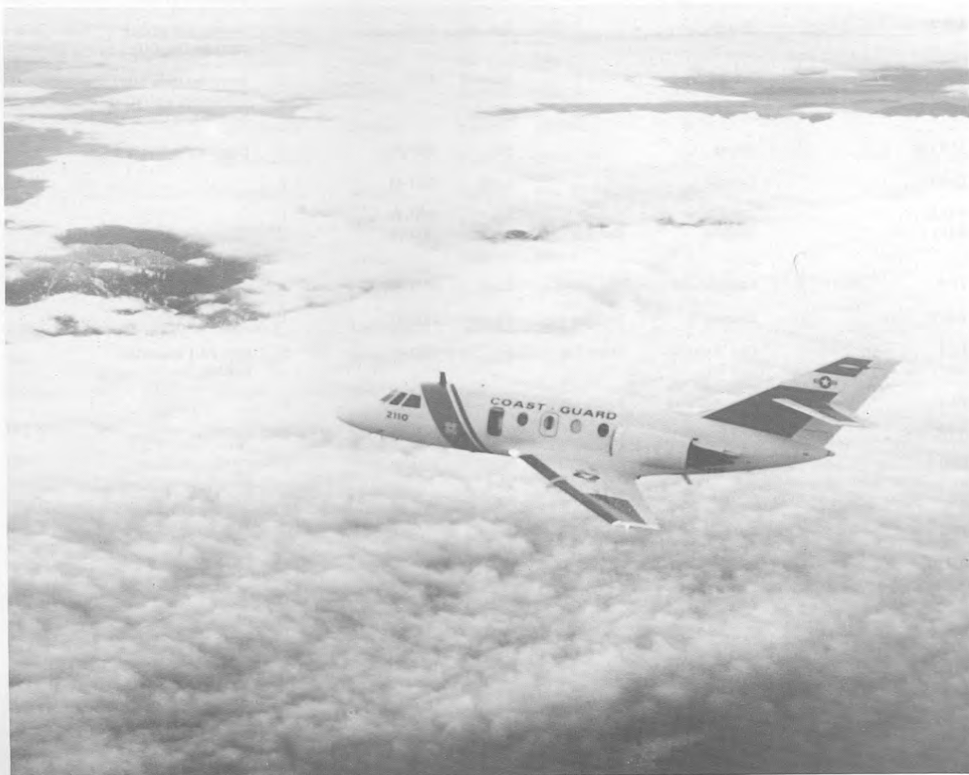
The HU-25A "Guardian", a new Coast Guard multi-mission jet, can operate from sea level to an altitude of 42,000 feet. Its 160-mile radius and five hour flight endurance make the Guardian a welcome addition to the Coast Guard's search and rescue and drug interdiction efforts.
