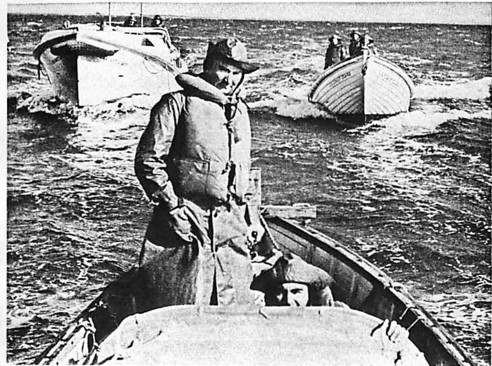
Motor lifeboat (left) and motor surfboat (right) are both self-bailing rescue craft.
