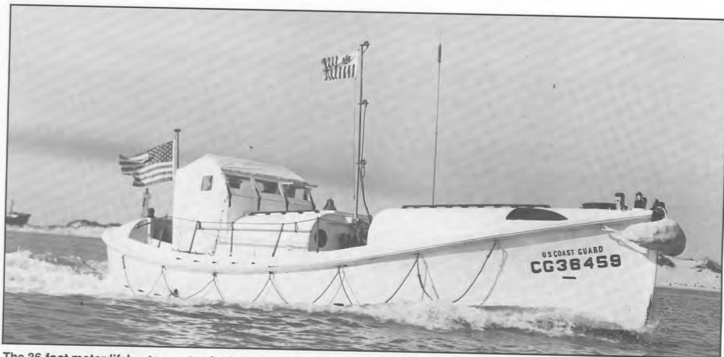
The 36-foot motor lifeboat was standard rough weather rescue craft in the Coast Guard from pre-WWII until 1962.
