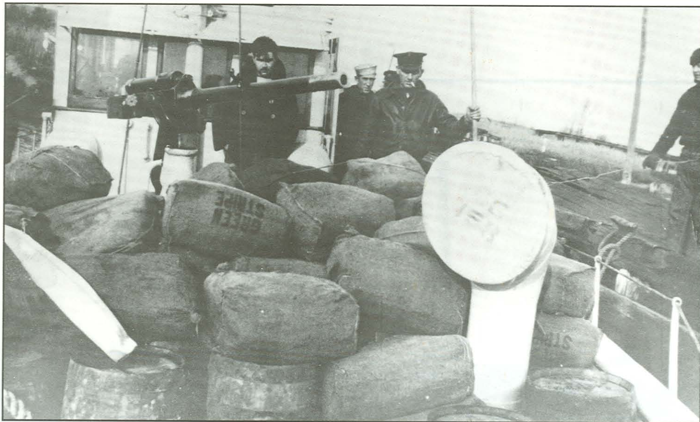
Crew of CG 158 looks over stash of illegal liquor which they had recently seized. Note that the liquor is packaged in burlap sacks. This was done to facilitate the loading and unloading by the rum runners. The single shot six-pounder just forward of the bridge was the principal weapon mounted on the "six bitters."
