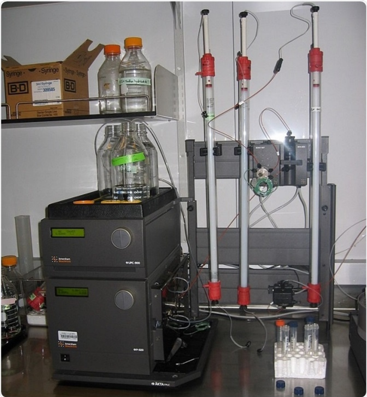
A laboratory set up of FPLC. Photo credit: Kjaergaard /commons.wikimedia.org
