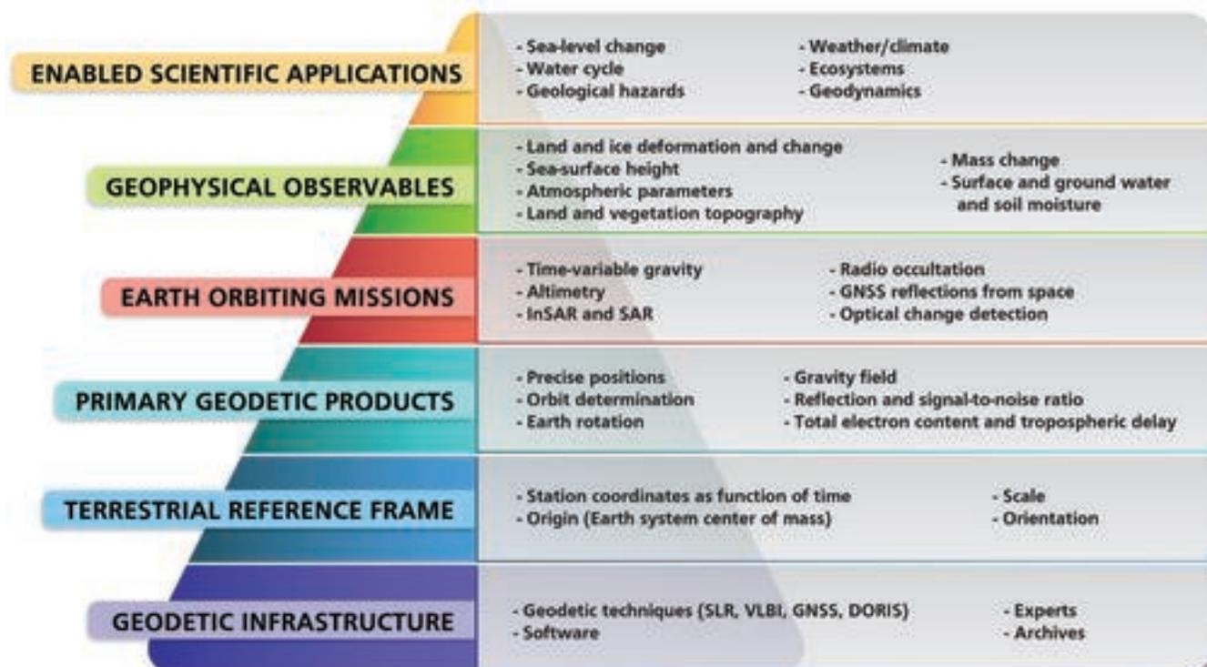
**FIGURE S.1** Illustration of how the geodetic infrastructure is connected to enabled scientific applications. NOTE: DORIS = Doppler Orbitography and Radiopositioning Integrated by Satellite; GNSS = Global Navigation Satellite System; InSAR = Interferometric Synthetic Aperture Radar; SLR = Satellite Laser Ranging; VLBI = Very Long Baseline Interferometry.
