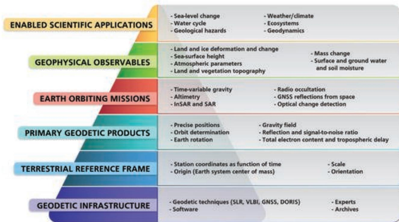
**FIGURE 1.1** Illustration of how the geodetic infrastructure is connected to enabled scientific applications. NOTE: DORIS = Doppler Orbitography and Radiopositioning Integrated by Satellite; GNSS = Global Navigation Satellite System; InSAR = Interferometric Synthetic Aperture Radar; SLR = Satellite Laser Ranging; VLBI = Very Long Baseline Interferometry.
