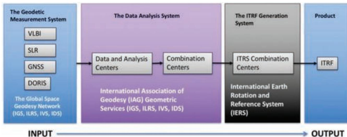
**FIGURE 1.5** Schematic diagram of the production of the ITRF using geodetic measurements from VLBI, SLR, GNSS, and DORIS. All of the associated geodetic services are organized under the International Association of Geodesy. NOTE: IDS = International DORIS Service; IGS = International GNSS Service; ILRS = International Laser Ranging Service; IVS = International VLBI Service for Geodesy and Astrometry. SOURCE: Frank Lemoine, NASA.
