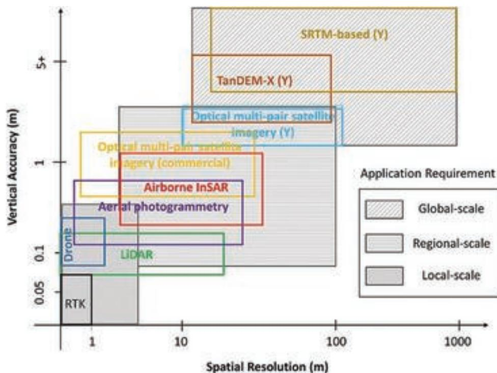
**FIGURE 7.2** Sensors that provide digital elevation model data at varying spatial resolutions and vertical accuracies. NOTE: InSAR = Interferometric Synthetic-Aperture Radar; LiDAR = Light Detection and Ranging; RTK = Real-time Kinematic; SRTM = Shuttle Radar Topography Mission; TanDEM-X = TerraSAR-X's twin satellite. SOURCE: Schumann and Bates, 2018.
