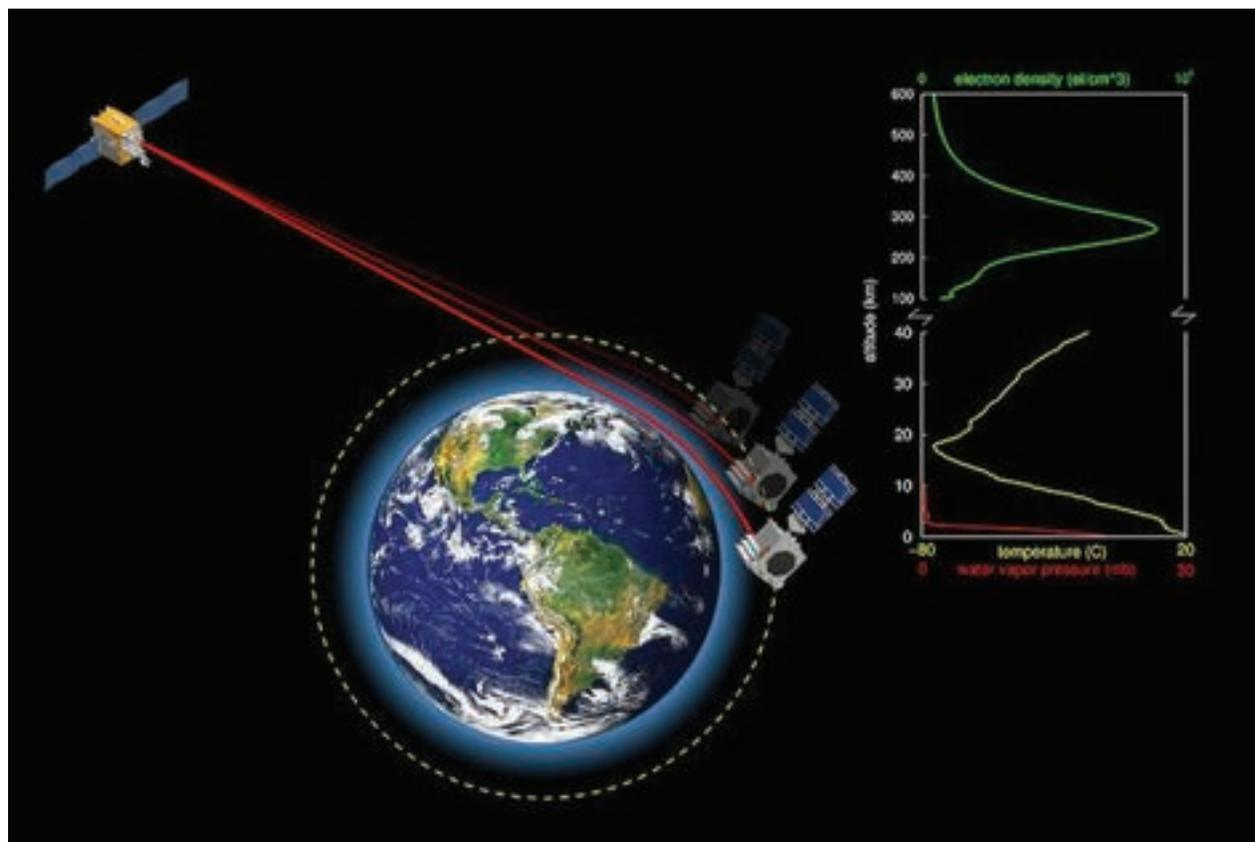
**FIGURE 6.1** Geometry of limb sounding GNSS-RO measurements to measure atmospheric profiles of temperature (yellow), water vapor pressure (red), and electron density (green). SOURCE: <https://www.cosmic.ucar.edu/what-we-do/cosmic-2>.
