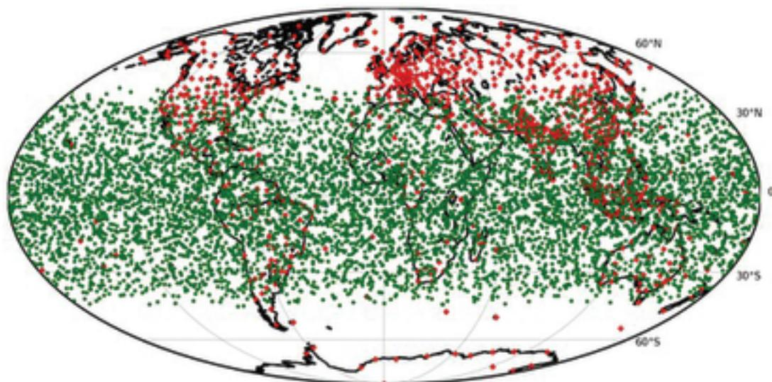
**FIGURE 6.3** Locations of 4,000 occultations (green) for the COSMIC-2 constellation of 6 GNSS receivers orbiting at an altitude of 500 km and an inclination of 24°. Ground-based radiosonde locations (red) only sample the atmosphere above land. SOURCE: <https://www.cosmic.ucar.edu/what-we-do/cosmic-2>.
