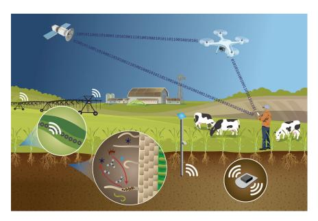
FIGURE 7-2 Schematic representation of real-time continuous monitoring of soil, crops, water, and livestock via microelectromechanical and biodegradable sensors. The sensors measure a range of important attributes to generate data. Data can then be analyzed and used for modeling and for predictive and prescriptive agriculture.
