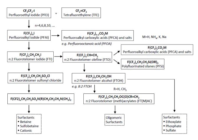
Figure A.B.2-1: Telomerisation process (figure based on (Knepper and Lange, 2012))
